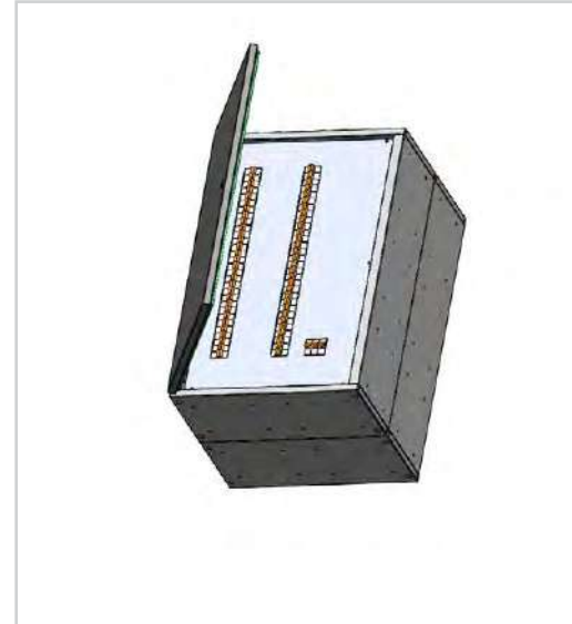
Cabinets can be nested on top of each other
