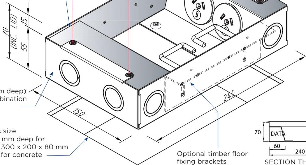
Nominal recess size 250 x 160 x 80 mm deep for timber floor or 300 x 200 x 80 mm foam blockout for concrete
